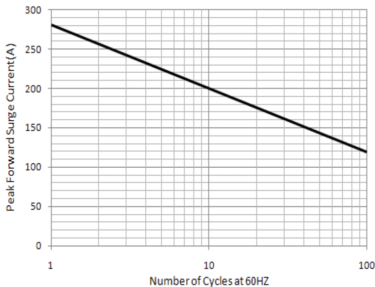
Figure 2. Maximum Non-Repetitive Peak Forward Surge Current Per Leg
